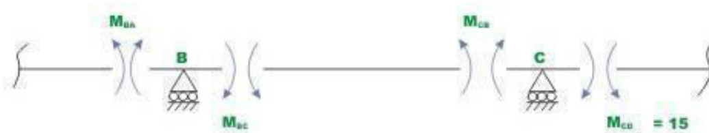
Fig. 14.6 b Free - body diagrams of joints B and C along with members
